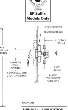
2"CC (51mm) 1 7/8" IPS (48mm) MAX WALL FACE OF STUD 1/2" MIN. CC (13mm) FINISHED WALL LINE 5/8" MIN IPS (16mm) 7-1/2" 2-5/8' (190mm) (67mm) 6.5" (165mm) 2 1/2" MAX. (63mm) ESC. DIAM. 6'-6" (1981mm) 4-1/2" (114mm) NOMINAL WALL OPENING DIRECTION OF HANDLE ROTATION 1-3/8" (35mm) SHOWER 45" (1143mm)/ 48" (1219mm) 5-1/4" (133mm) 32" (813mm) TUB/SHOWER AND TUB ONLY FLOOR LINE **TUB RIM** THICK WALL APPLICATION THIN WALL APPLICATION
