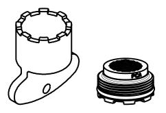
Aerator, Male Vandal Resistant 1.2 gpm (4.5L/min)
