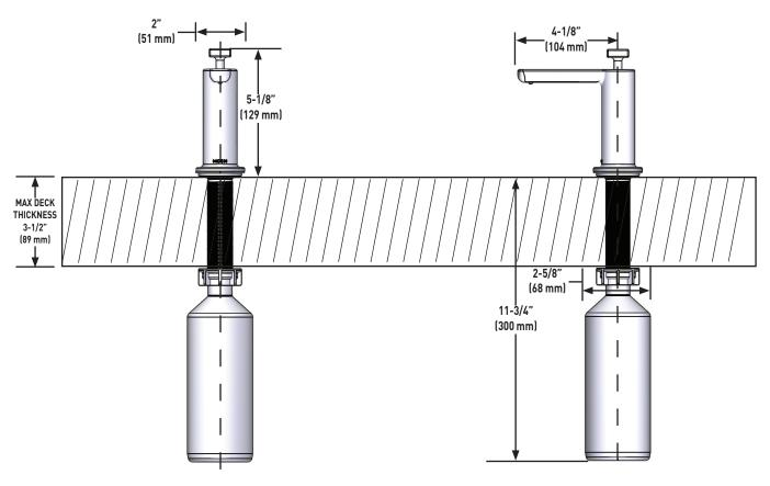
NOTE: DESIGNED TO BE INSTALLED THROUGH 1 HOLE 1-1/8" DIAMETER
