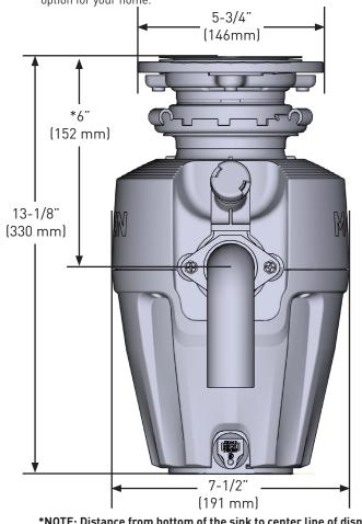
\*NOTE: Distance from bottom of the sink to center line of disposal discharge. Add 1/2" (13 mm) when a stainless steel sink is used.
