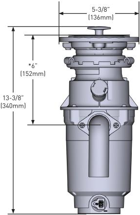
\*NOTE: Distance from bottom of the sink to center line of disposal discharge.
