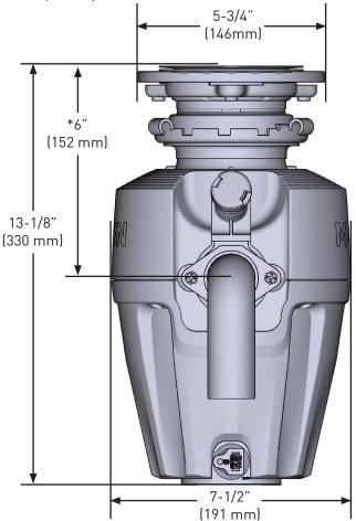
\*NOTE: Distance from bottom of the sink to center line of disposal discharge.
