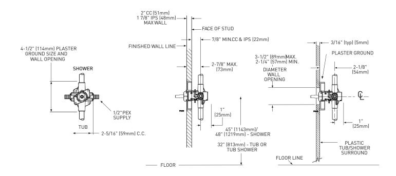
\* The PEX Posi-Temp valves are NOT to be used with polybutylene (PB) tubing or the Wirsbo "expandable" joining system
