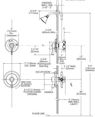
NOTE: This valve is not intended to be used as a shut-off valve. To prevent the potential of cross flow, check valves must be integral to the supply valve or installed in both hot and cold water supply lines.
