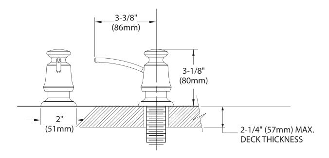
**NOTE:** DESIGNED TO BE INSTALLED THROUGH 1 HOLE 1-1/8" DIAMETER
