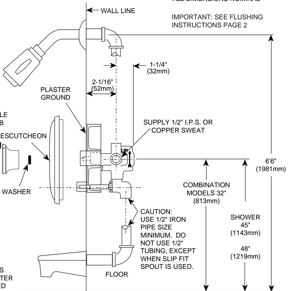
CAUTION: USE 1/2" IRON PIPE SIZE MINIMUM. DO NOT USE 1/2" TUBING, EXCEPT WHEN SLIP FIT SPOUT IS USED.
