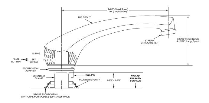
Open trim package and check to see that all parts for the tub filler installation have been enclosed:
