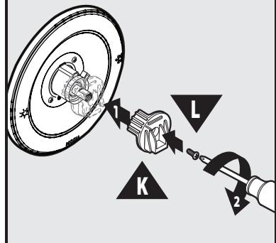
Remove the Lever (M) and Lever Handle Adapter (K). Note the position on the stop. Position the Adjustable Temperature Limit Stop (D) so the Lever stops at the position. This prevents the Lever from being turned into an unsafe temperature.
