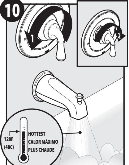
Turn handle on to test hot water temperature. Turn off handle if desired water temperature has been met. Hot water temperature should not exceed 120°F.
