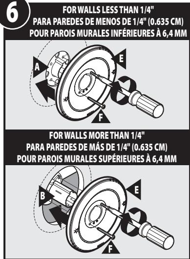
Secure Escutcheon (**E**) against wall by threading Screws (**F**) through Escutcheon into valve.
