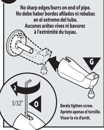
No sharp edges/burrs on end of pipe.
