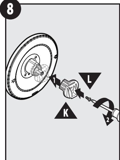
Install Handle Adapter (**K**) onto cartridge stem with Handle Adapter Screw (**L**).
