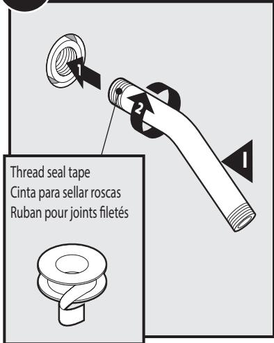
Wrap thread seal tape around Shower Arm (I) threads. Screw Shower Arm into connection in wall.
