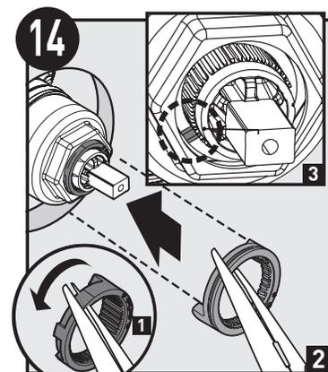
Install the adjustable temperature limit stop so it is in contact with the bottom of the stop on the left side of the cartridge, as shown in inset.
