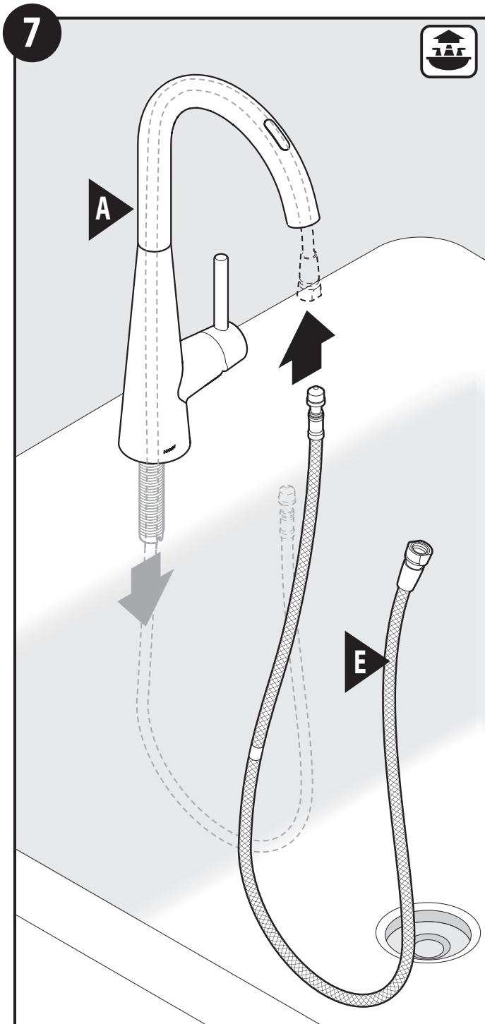
Insert small end of pulldown hose (**E**) into spout and feed through faucet body (**A**).
