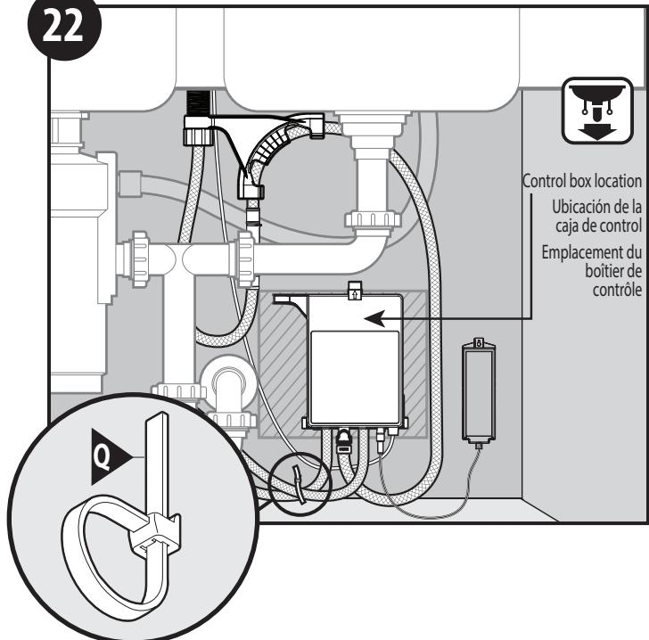
Use zip ties (Q) if desired to manage faucet hoses, data cable and battery holder cable. **Do not zip tie pulldown hose.** Check to ensure pulldown hose movement is not obstructed.
