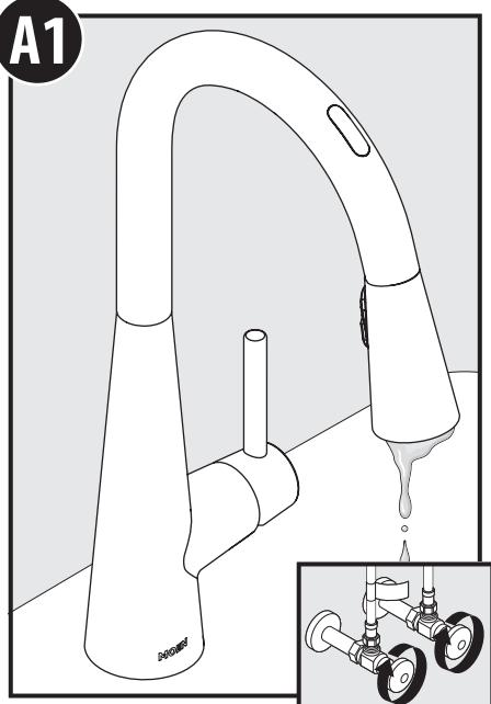
If low flow, turn off water at stops before cleaning filters.
