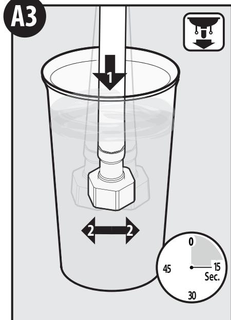
1. Insert each filter hose into a cup of water.
