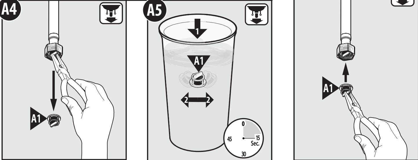
**Note:** Filter screen (A1) can be removed for further cleaning. Screen must be reinstalled to maintain product warranty. Use fingers or needle nose pliers to remove Filter Screen (A1).
