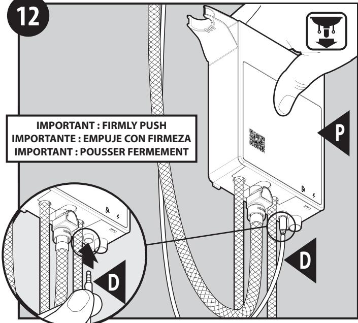
Insert data cable (**D**) to data port on bottom of control box (**P**). Ensure cable is pushed all the way into the control box.
