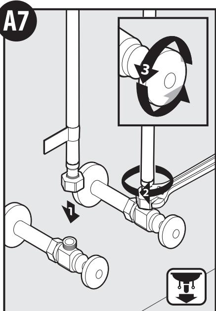
1. Connect supply lines to shut off valves. Ensure faucet supply line with label connects to the hot supply stop.
