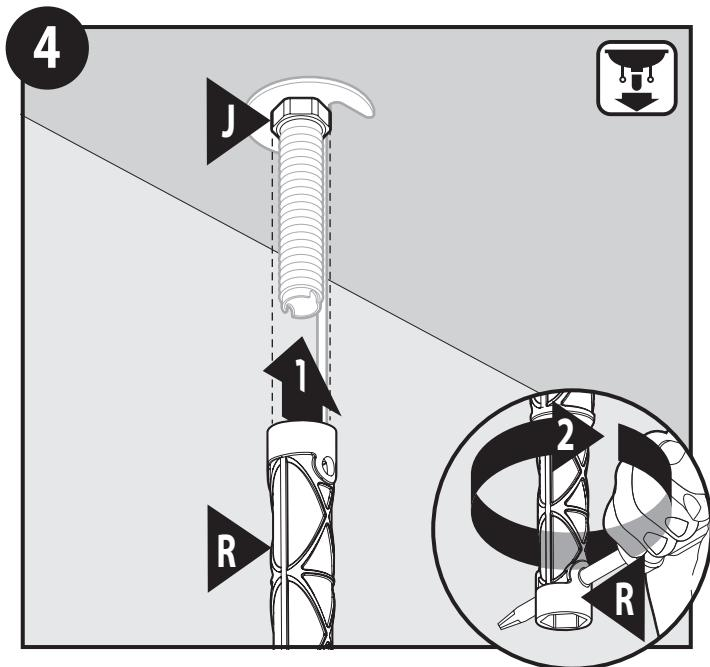
1. Tighten mounting nut (J) with installation tool (R).
