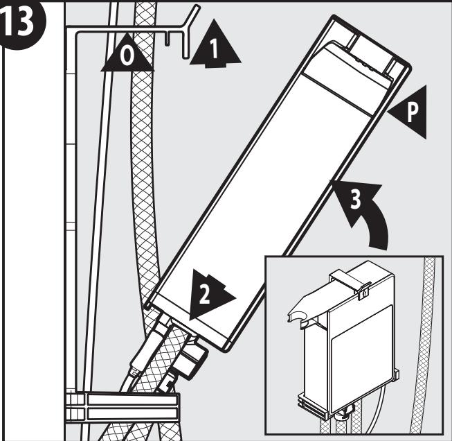
1. Lift tab of Wall Mounting Bracket (**O**).
