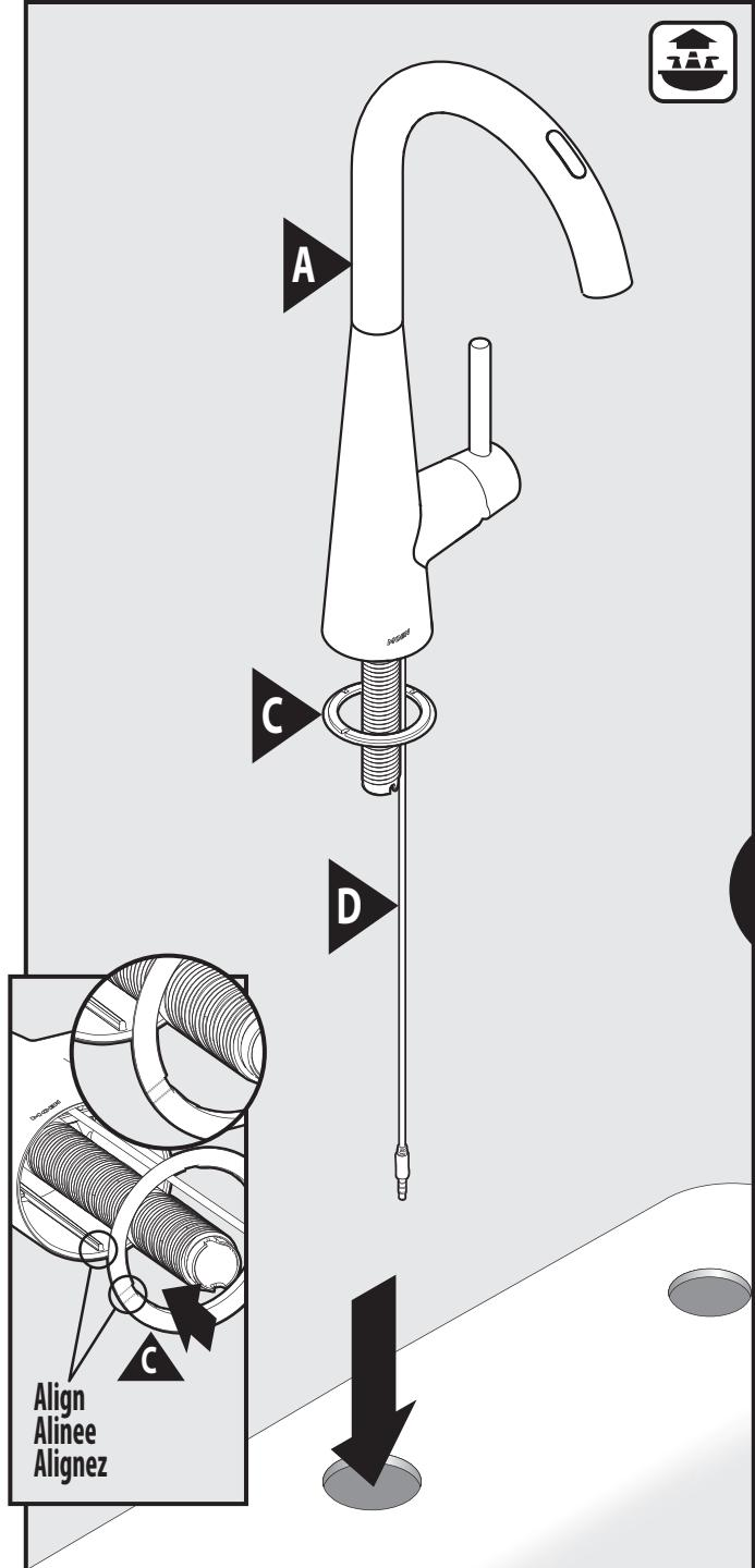
Install faucet body (A)—including data cable (D), and single hole deck gasket (C)—in hole on sink. **Note:** Installs with handle on right side only.
