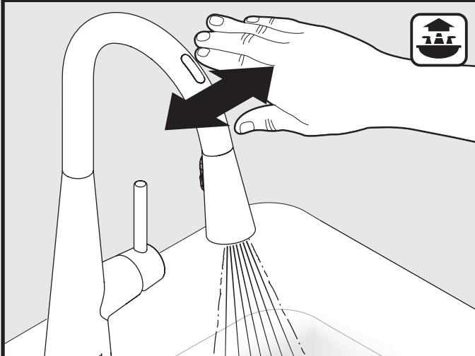
Check to ensure wave sensor is working properly. Move hand over wave sensor to test that water will turn on. Move hand over wave sensor again to turn water off. If water does not flow properly, see trouble shooting section on page 20.
