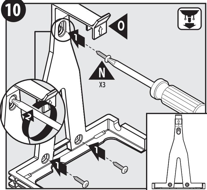
Secure Wall Mounting Bracket (O) to wall with provided Mounting Screws (N). If installing into dry wall, use appropriate anchors and screws (not provided).
