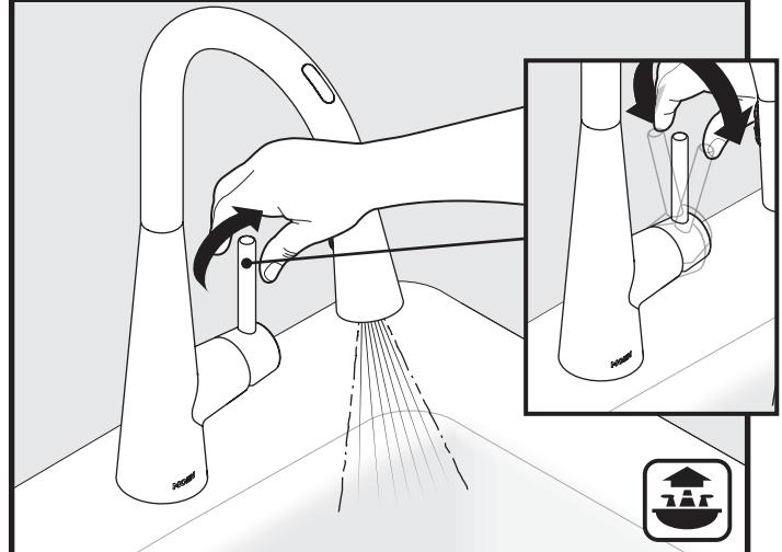
Check to ensure handle is working properly. Turn on water with handle to test that hot and cold water will run. Turn handle off. If water does not flow properly, see trouble shooting section on page 20.
