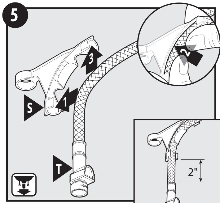
Install pulldown connecting hose bracket (S) onto lower end of extension hose (T), about 2"
