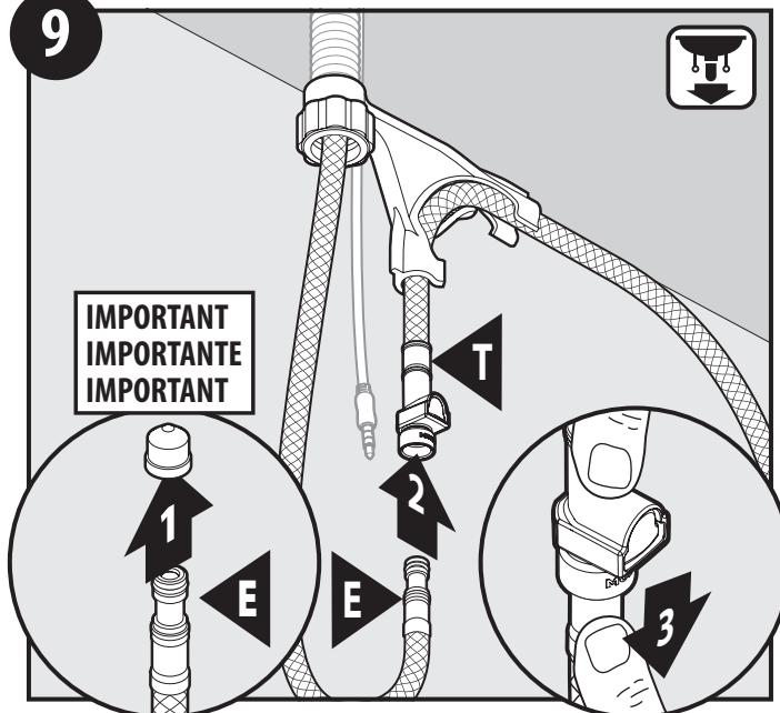
1. Remove and discard protective cap from pulldown hose (E).
