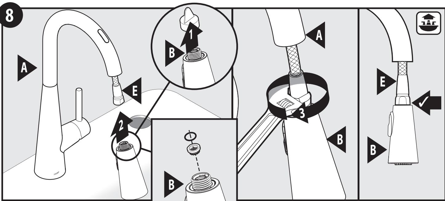
1. Remove and discard protective cap from spray wand (B). (*Ensure o-ring and screen are in place.*)
