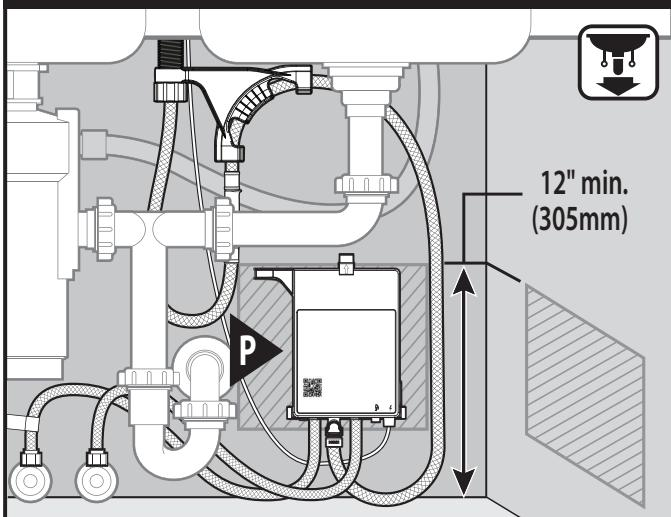
**For easier serviceability, mount control box minimum 12" (305mm) above floor.**
