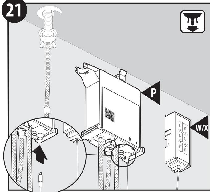
Insert battery holder (W/X) cable into control box (P) power port. Ensure cable is pushed all the way into the control box.
