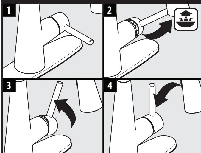
In order to help the faucet achieve optimal performance, you will need to help calibrate it to your homes unique specifications. To do this, you will need to move the handle around in a full circle. Start with the faucet in the closed full cold position, then open it to full cold, move the handle up to the full hot position and then close it in the full hot position. It's important to wait a few seconds during each step.
