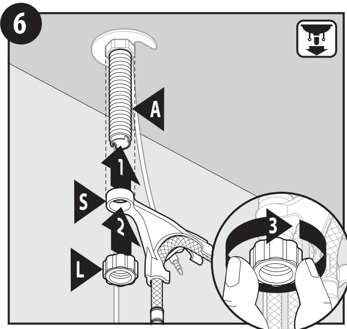
Slide pulldown connecting hose bracket (**S**) over threaded shank and secure with hose protector (**L**).
