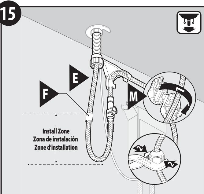
Locate hose weight locator mark (**F**) on pulldown hose (**E**). **1.** Install hose weight (**M**) just above start of loop curvature in hose on the same side of hose as locator mark (**F**). **2.** Pliers can be used for installation assistance.
