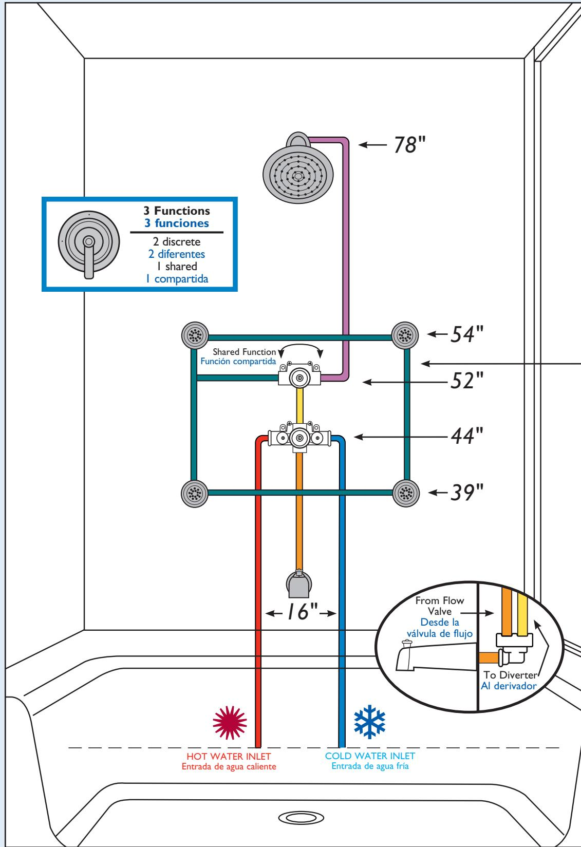
When using a tub spout with a mixing valve and diverter, plumb the flow valve bottom outlet to the twin ell front vertical inlet. Plug the top outlet of the flow valve. Plumb the twin ell rear vertical outlet to the diverter. Plumb the twin ell front horizontal outlet to the tub spout.
