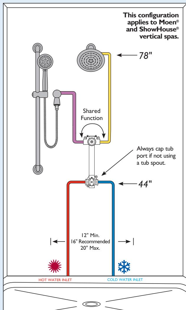
All vertical dimensions (*italicized*) measured from floor.
