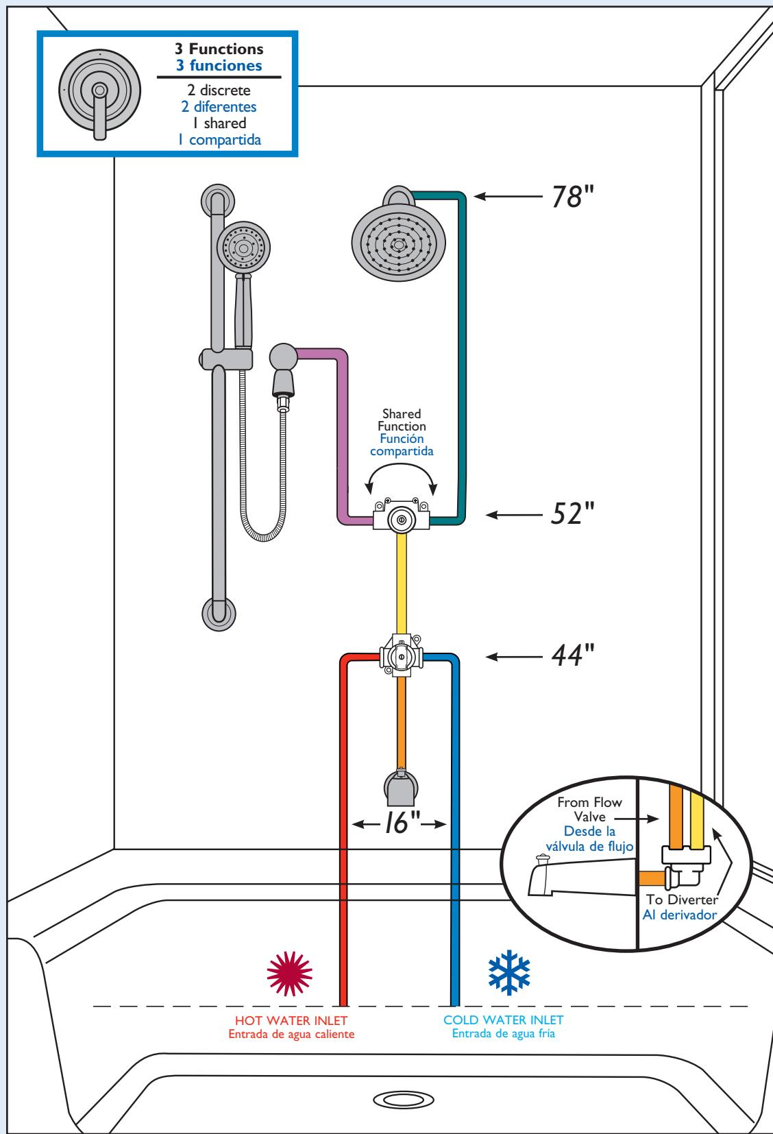
All vertical dimensions (*italicized*) measured from floor. Dimensions listed are suggested.
